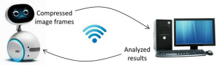
Figure 1: System architecture. Due to the limited computational resources available on a robot, we extend them by a high-performance computer. We transmit data between the robot and the computer via the wireless connection to ensure the robot’s moving capability.
