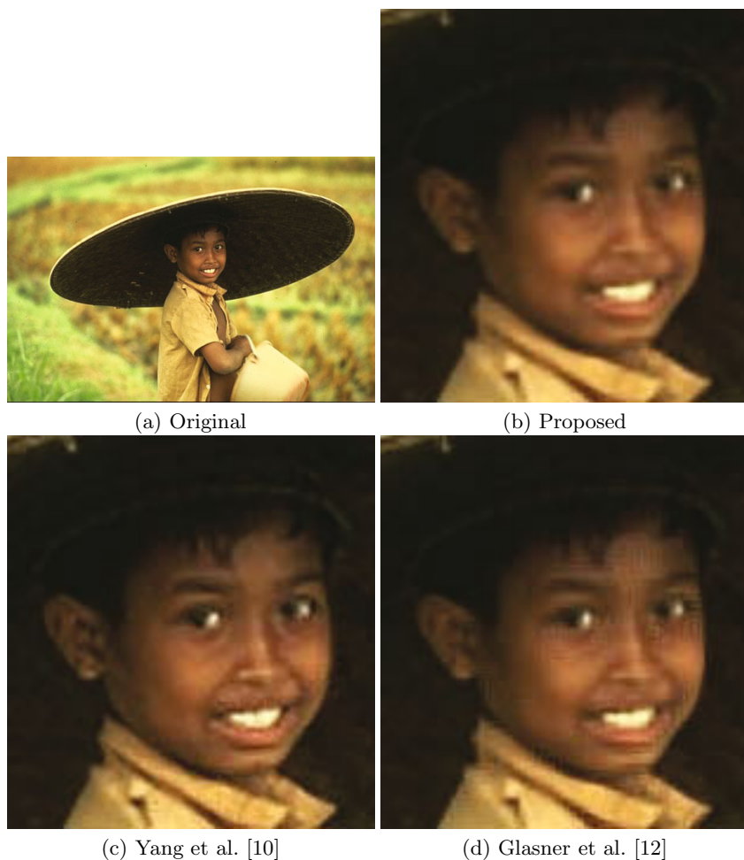
Fig. 6. Boy (results best viewed on a high-resolution display). Compared with result generated by [12], our super-resolution image has fewer artifacts (e.g., several blotches in the facial and collar regions). Compared with result generated by [10], our super-resolution image has fewer artifacts (e.g., several large blotches in the lip and contour regions).
